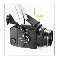
2) To attach Prism Finder S, align the front end of the finder with the front end of the finder frame (the shiny square frame on top of the camera body). Then, gently lower the finder and, when well seated, slide forward until it locks.
