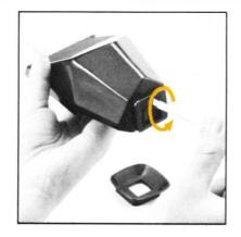
2) To exchange eyepiece lens, first, detach the eyecup. Then, unscrew the setscrew on the eyepiece lens frame and it will be possible to remove the lens together with the frame.
